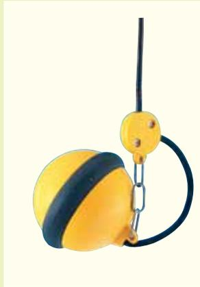
Model RF-5 is an economy type float which can detect upper/lower-limit water levels with single float. The snap on-off action ensures stable operation in clean or waste water containing suspended solids or oil and fat.
