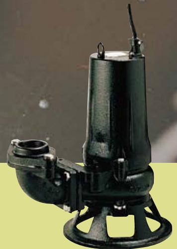
**The C-series incorporates a cutter mechanism consisting of a tungsten carbide tipped channel impeller and a saw-tooth suction cover surface hardened. The cutter mechanism cuts fibrous materials to small pieces permitting clog-free pumping.**
