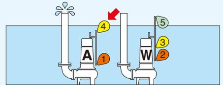
1 Start float 4 of pump A operates to start water discharge.
