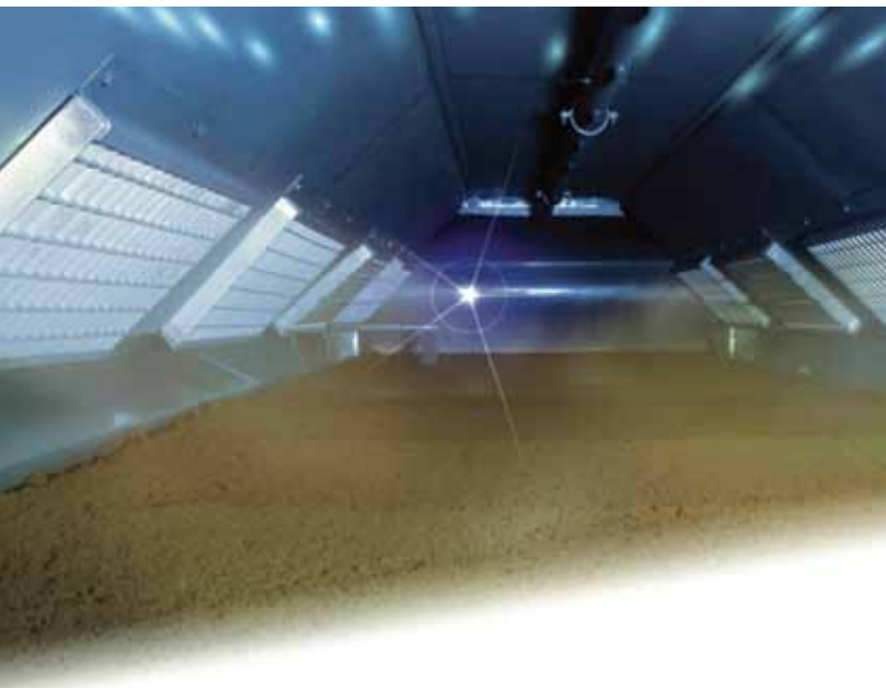
Belt dryer for sludge
