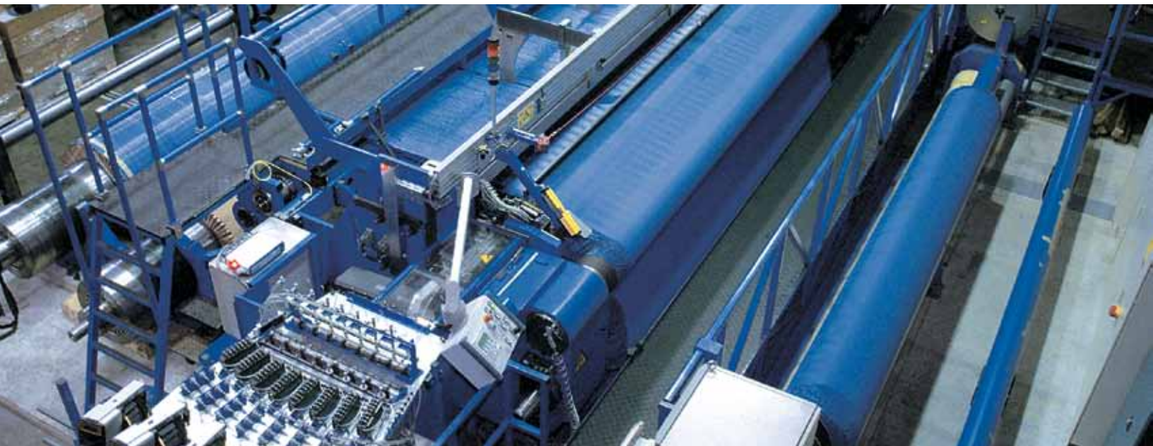
Loom for plastic woven belts with seven meters working width
