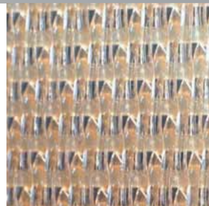
PPS 5099 mesh for high chemical or thermal load
