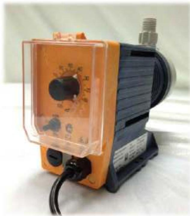
The Prominent super dose is a micro processor controlled short stroke solenoid operated diaphragm metering pump for liquid Metering is based pulsating action. For each pulse come from electronic control the solenoid energizes and completes stroke .The diaphragm stabilized by a steel core displace medium the liquid end the ball on delivery side open thus releasing the medium for metering .
