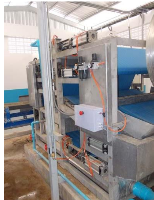
Automatic belt tracking alignment & Tension control Belt variable speed control
