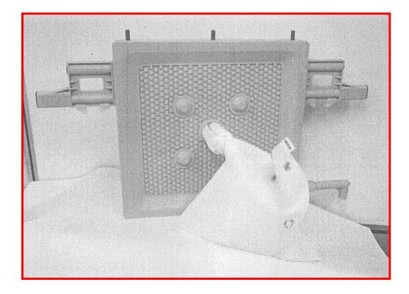
Put both ends at the same time into the center feed hole and pull from the opposite side as shown.
