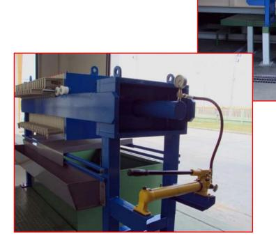
Manual hand hydraulic pressing device Manual plate opening type
